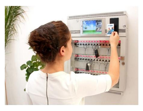
The KeySafe Lock is a safety key-storage cabinet, that can be opened only with personal RFID proximity card (transponder) or/and with a PIN code, optionally using fingerprint identification, if the device is a KeySafeLockBio. The offline type has an inbuilt computer. It is possible to connect it to a computer network and to check remotely who and when took which key and for how long time.
